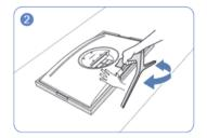
To disassemble the stand from the monitor, be sure to press the lower part of the monitor with one hand, and shake the stand from side to side with the other hand to make some gap between them.
