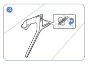
Tightly fasten the connecting screw at the bottom of the stand base.
