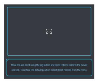
1 The aim point is displayed in the middle of the screen. Position adjustment is only possible within the displayed rectangular area.
