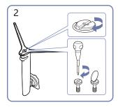
Tightly fasten the connecting screw at the bottom of the stand base.
